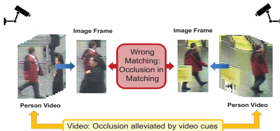
Figure 1. Video instances vs. still-image instances of the same person. It is clear that video contains much richer cues for matching.
