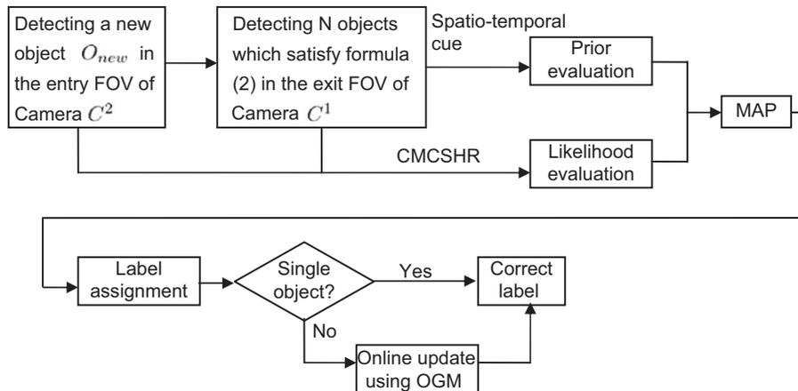
Fig. 2. The Bayesian model approach for consistent labeling across two non-overlapping camera views.
