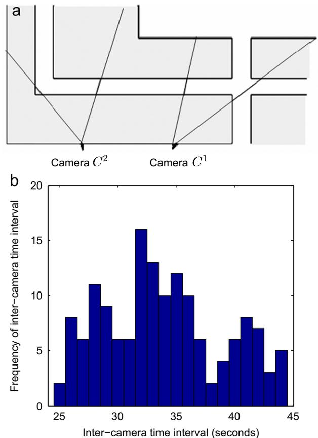
**Fig. 10.** (a) Camera configuration for the first experiment (scenario 1). (b) The histogram of the inter-camera time interval (learned from training data). Note that most people take almost 35 s to walk from camera  $C^1$  to camera  $C^2$ ; the minimum time is about 25 s and the maximum time is about 45 s.
