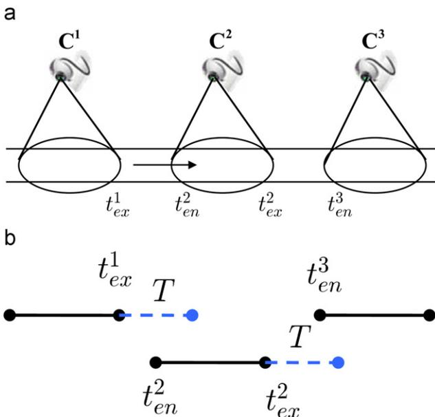
Fig. 1. An example of camera setup and their temporal relationship in multiple non-overlapping camera views: (a) Camera setup. (b) Temporal relationship between camera views. See text for details.
