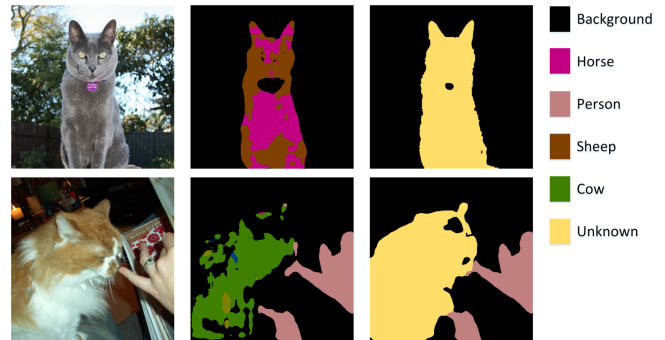
Fig. 1. Examples of open set semantic segmentation. Left column: input images in which regions of cat belongs to the unknown class; Middle: segmentation results in close set semantic segmentation where any unknown region was forced to be segmented into known class(es); Right: open set semantic segmentation result based on the proposed method.
